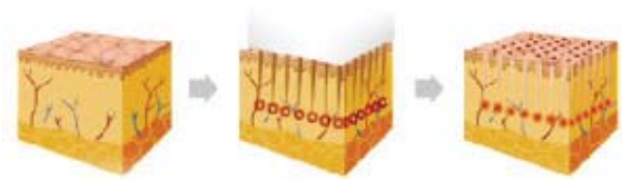
Fig 5: First pass with the INFINI. The needles enter the skin, deliver the RF energy (center) and withdraw, leaving a discrete zone of dermal damage at the preset depth (right).
